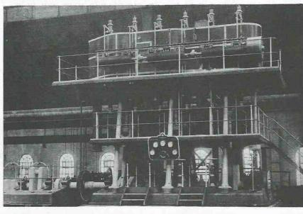
The Chelvey triple-expansion engine assembled for testing at Lilleshall works
