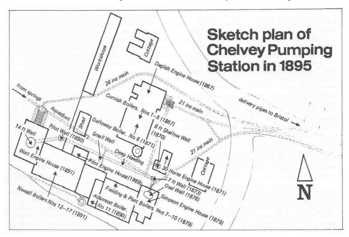
but in fact flooded his works from the higher level there. The 30 horse engine was started, coupled to the 14 in pumps in the 7 ft well but could lower the water no more than 11 ft.
